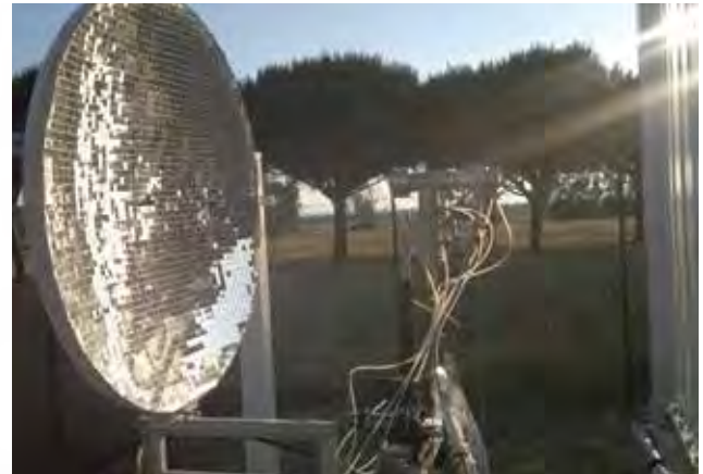
Fig. 3. The conversion module CM installed on the parabolic concentrator focus.
