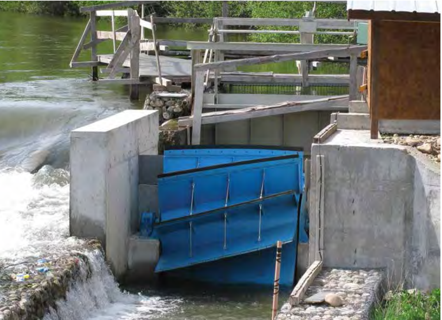
Fig. 1: Hydrostatic Pressure Machine, Prototype River Iskar / Bulgaria
