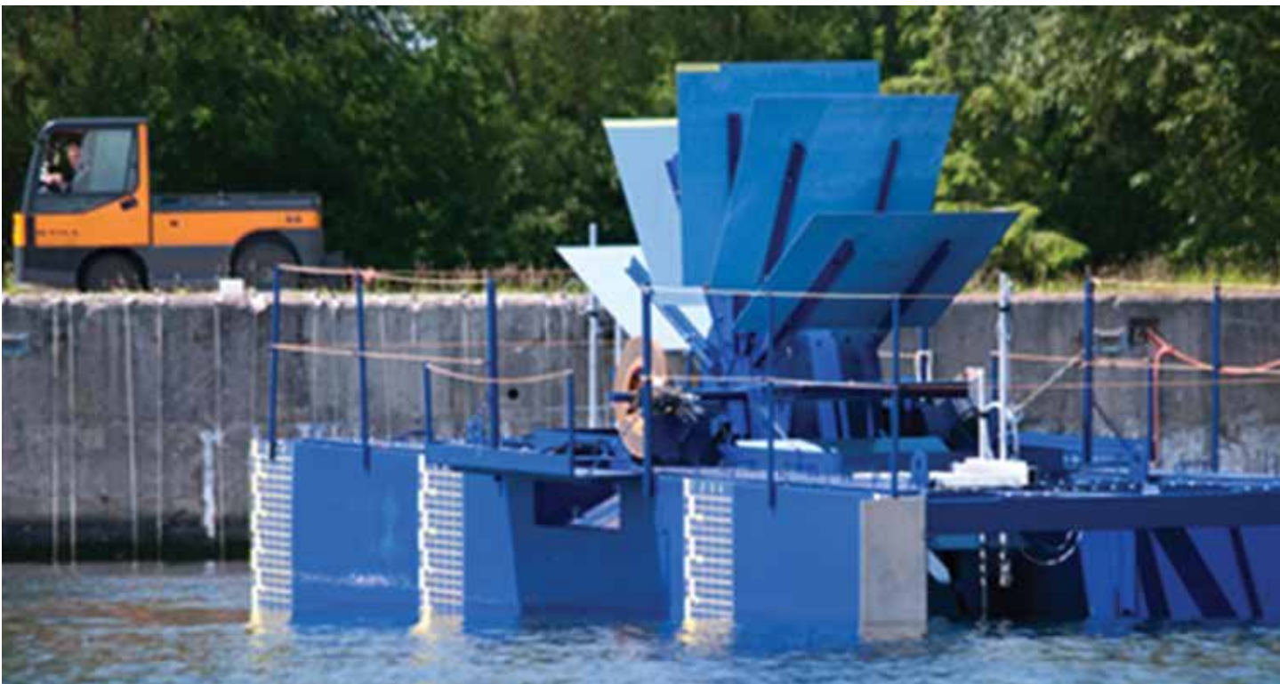
Fig. 2: Free Stream Energy Converter for exploitation of river currents
